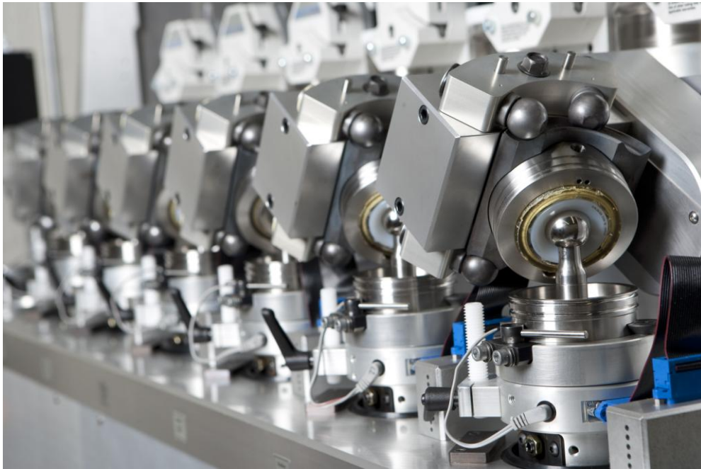
One six-station bank of the ADL Hip Simulator
